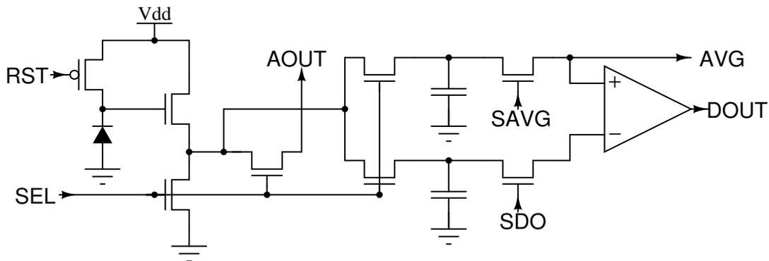
Figure 2: Custom active pixel sensor (APS) Cell
