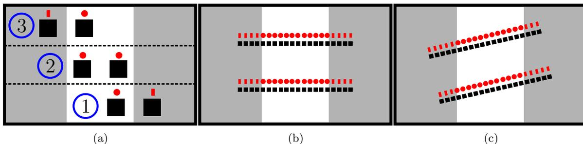
Figure 1: ■ = sensor; ■ = high level; ● = low level; (a) Two-sensor configuration; (b) Two 32-pixel length array aligned with the path; (c) Misalignment of the path is detected as a difference between the lateral pixel of each array.
